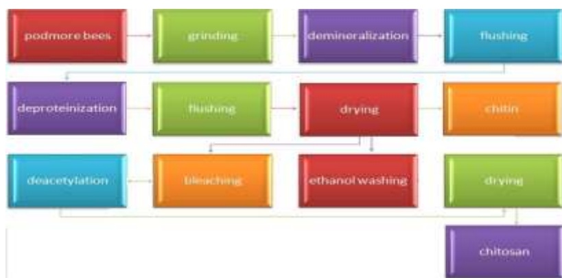
Figure 3. Outline scheme for the production of chitin and chitosan
